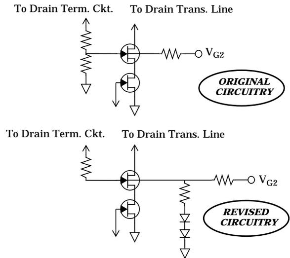
Figure 2. HMMC-5021/22/26  $V_{G2}$  Circuitry Changes
