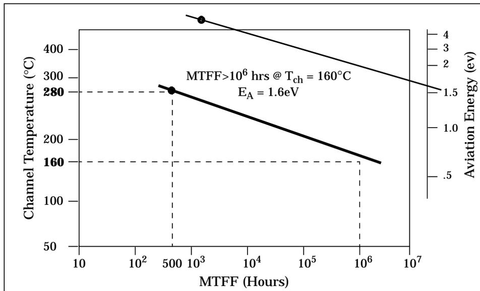
Figure 1. HMMC-5040 Arrhenius Plot
