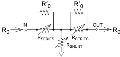
**Figure 4. HMMC-1002 Simplified Schematic**
