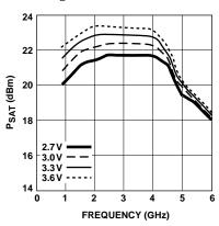
Figure 5. Saturated Output Power (+4 dBm in) vs. Frequency and Voltage.
