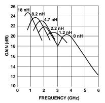
Figure 17. Available Gain (G<sub>max</sub>) vs. Frequency for the MGA-83563 Amplifier over Various Inductance Values.
