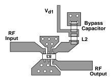
Figure 21. Basic PCB Layout.
