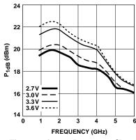
Figure 4. Output Power at 1 dB Compression vs. Frequency and Voltage.
