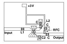
Figure 28. Completed 2.5 GHz Amplifier Assembly.
