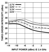
Figure 13. Third Order Intercept vs. Input Power and Voltage. Note: Figure 1 test circuit.
