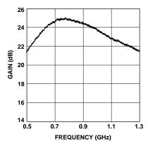
Figure 35. Small Signal Gain of the 900 MHz Amplifier.
