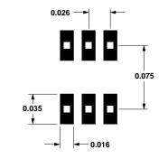
Figure 20. PCB Pad Layout for MGA-83563 Package (dimensions in inches).
