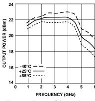
Figure 7. Saturated Output Power (+4 dBm in) vs. Frequency and Temperature.
