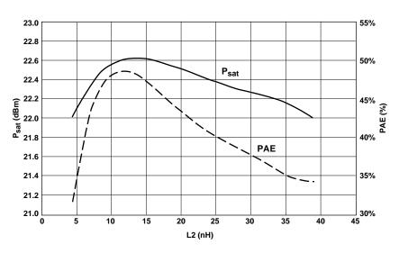
Figure 37. 900 MHz Psat and PAE vs. L2.
