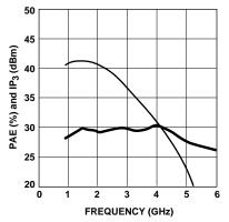
Figure 14. Power Added Efficiency and Third Order Intercept vs. Frequency  $(V_d = 3.6 V)$ .
