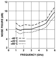
Figure 8. Noise Figure vs. Frequency and Temperature.
