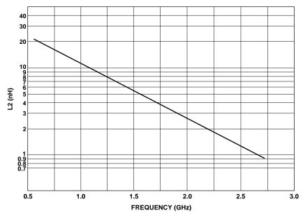
Figure 19. Values for Interstage Inductor L2.
