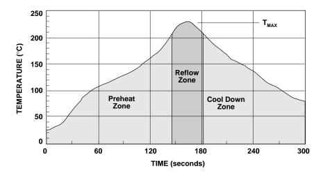
Figure 44. Surface Mount Assembly Profile.
