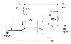
Figure 18. Interstage Inductor L2 and Bias Current.
