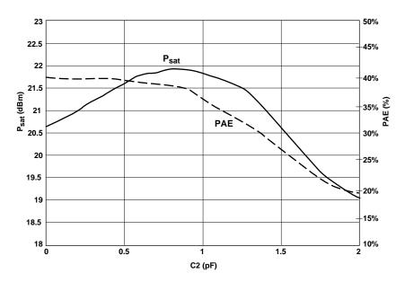
Figure 32. 2.5 GHz Psat and PAE vs. C2.
