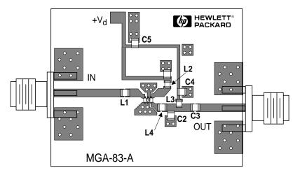
Figure 39. Completed MGA-83563 Amplifier Assembly.
