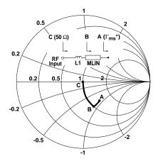
Figure 25. Initial Small Signal Input Match.
