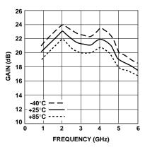
Figure 6. Gain vs. Frequency and Temperature.
