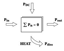
Figure 22. Thermal Representation of MGA-83563.
