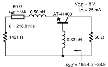
Figure 5. Dielectric Resonator Oscillator (DRO) at 4 GHz
