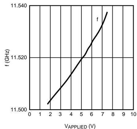
**Figure 7. Test Data for 11.5 GHz DRO**
