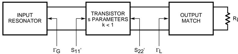
**Figure 1. Oscillator Design**
