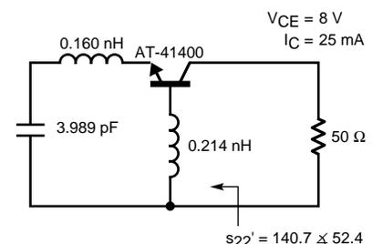
Figure 3. Lumped Resonator Oscillator at 4 GHz
