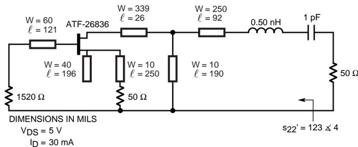
Figure 6. Dielectric Resonator Oscillator (DRO) at 11.5 GHz
