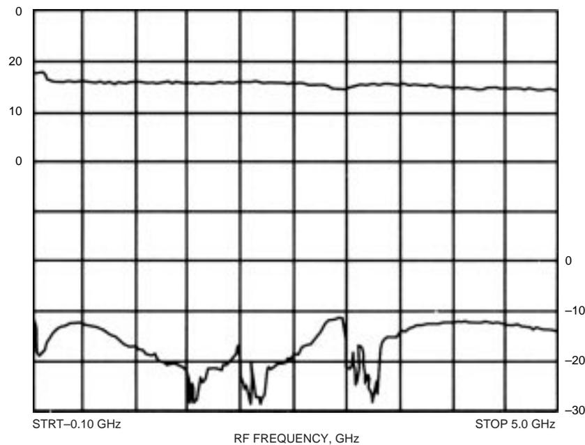
**Figure 11. Conversion Gain and Input Return Loss vs. Frequency, IAM-82028, I<sub>d</sub> = 56 mA, F<sub>IF</sub> = 100 MHz**
