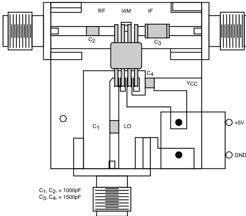
**Figure 9. IAM-8 Mixer Demonstration Circuit Showing Component Placement**
