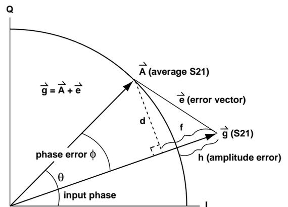
Figure 2. Illustration of error vector magnitude for calculating percent modulation error.
