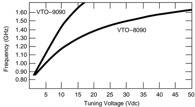
**Figure 12. Tuning voltage vs. frequency for similar non-buffered VCO modules. One uses an abrupt-tuning varactor, the other a hyperabrupt-tuning varactor. The hyperabrupt varactor provides a significant improvement in tuning linearity with a significantly lower tuning-voltage range.**
