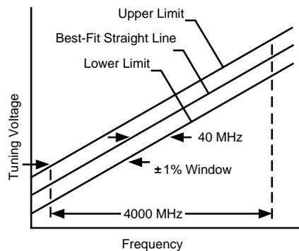
**Figure 16. The tuning curve of a linearized VCO will fall within a window about a straight line. "Percent linearity" is the term used to define the actual linearity achieved vs. the "best-fit straight line." Within the window there will be typically some irregular variations in slope due to the breakpoints in the linearizer.**
