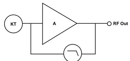
**Figure 1. Block diagram of a microwave oscillator, modeled as a combination of an amplifier with a positive-feedback loop and a frequency-determining network. KT represents the noise input that starts oscillation.**
