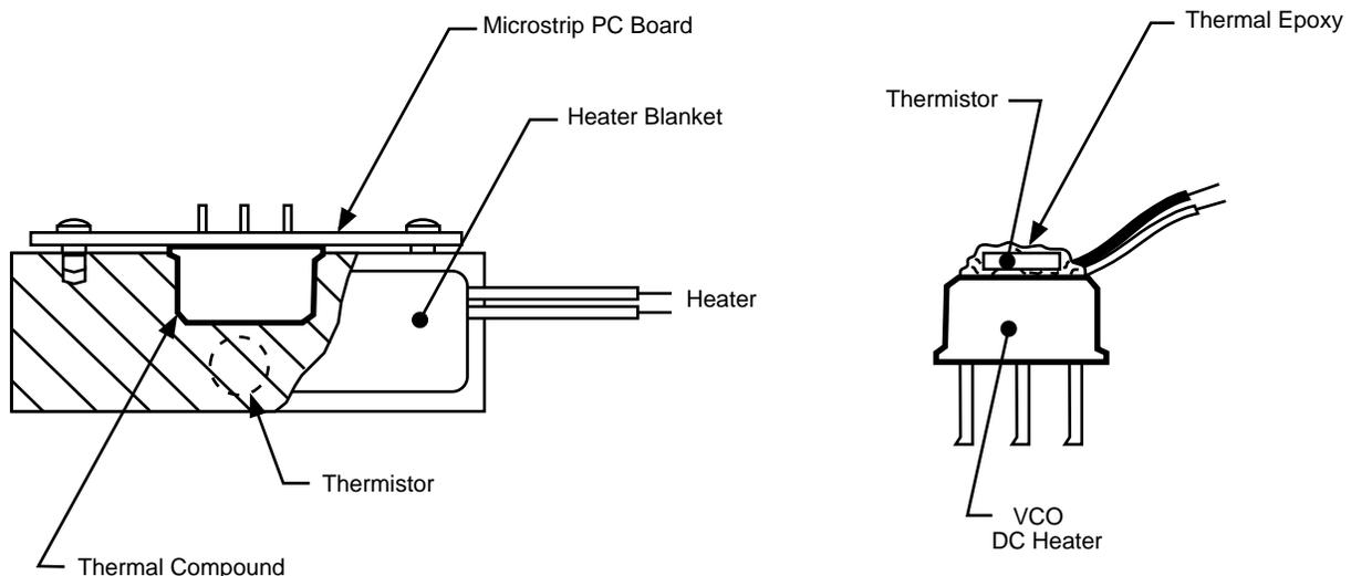
**Figure 21.** The temperature of a small VCO may be stabilized by mounting the oscillator on a block (which provides thermal mass) that is temperature-controlled by using a proportional heater, or with a small heater directly epoxied to the top of the TO-8 oscillator.
