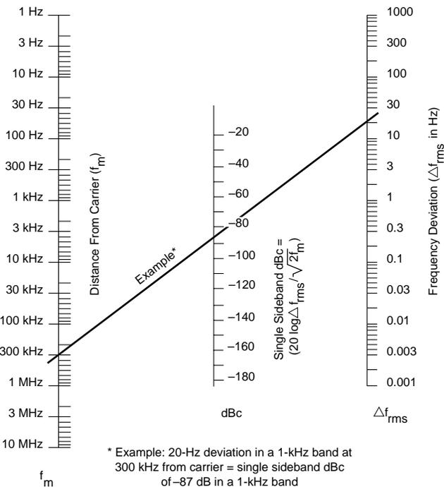
**Figure 6. FM noise-conversion nomograph. By placing a straight edge on the frequency deviation in Hz (right column) and on the distance from the carrier at which that deviation occurs (left column), the single-sideband noise-power ratio in dBc is shown in the center column.**
