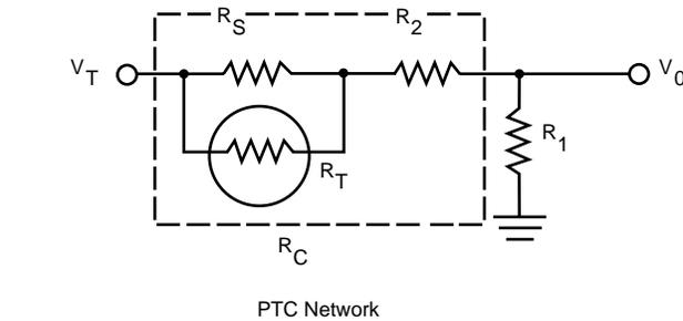
$$V_0 = (V_T R_1) / [R_1 + R_2 + (R_S \parallel R_T)]$$
