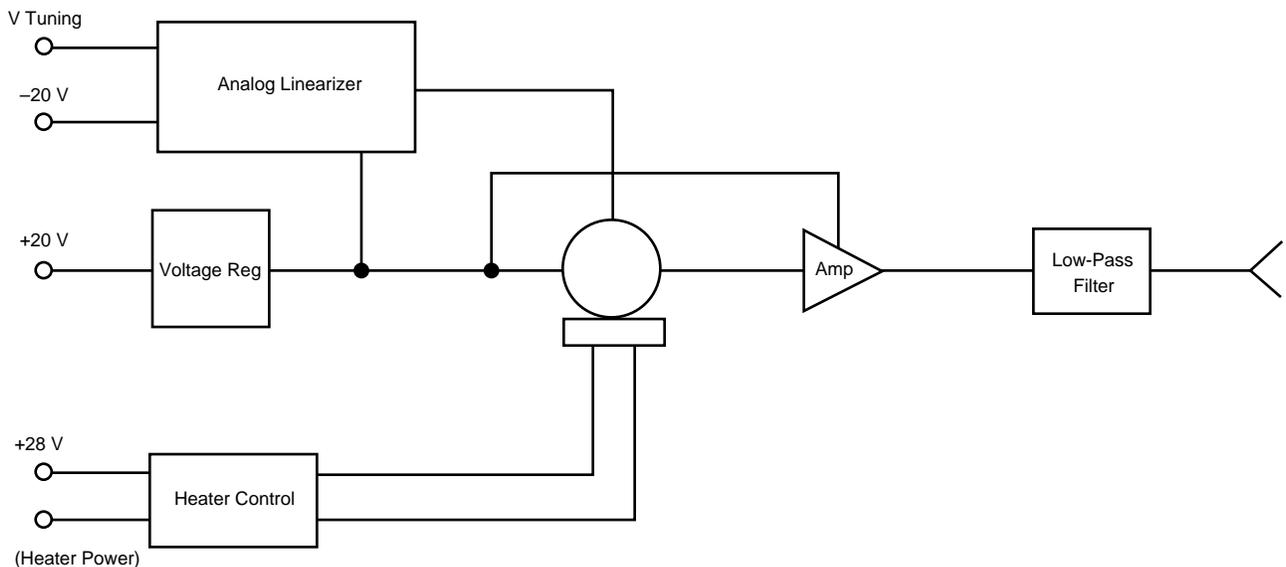
**Figure 24. A typical VCO assembly integrates a voltage-controlled oscillator with amplifiers, voltage regulators, linearizer, and heater circuitry. Typical VCO assembly specifications are given in Table II.**
