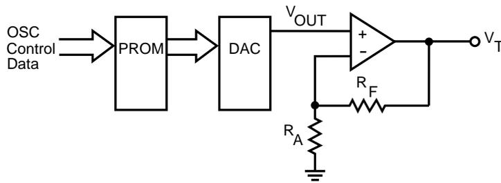
**Figure 20.** One of the most efficient linearization techniques combines an analog-to-digital converter with a PROM and an op amp. The PROM may be programmed to provide linearity better than 0.5% across the full frequency spectrum of the VCO and will also provide extremely fast tuning-response time, primarily limited by the settling time of the op amp.
