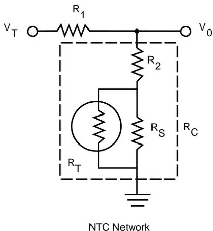
$$V_0 = V_t (R_2 + R_s \parallel R_T) / [R_1 + R_2 + (R_s \parallel R_T)]$$
