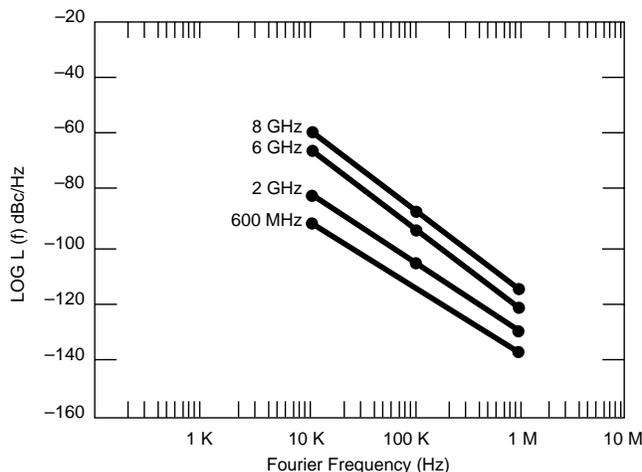
**Figure 7. Single-sideband phase-noise comparison of four production VCOs.**
