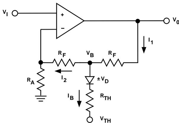
Figure 17. In this typical analog-linearizer circuit,  $V_{TH}$  will determine where an increase in the voltage-vs.-frequency slope will occur and  $R_{TH}$  will determine the amount of the increase in the slope that takes place.
