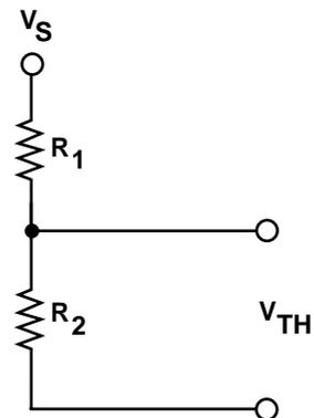
Figure 19. To replace  $R_{TH}$  and  $V_{TH}$  (Figs. 17 and 18) with a simple resistive divider, it is possible to calculate the required values using Thevenin's theorem. This provides the capability of introducing almost any number of changes to the slope of the tuning curve.
