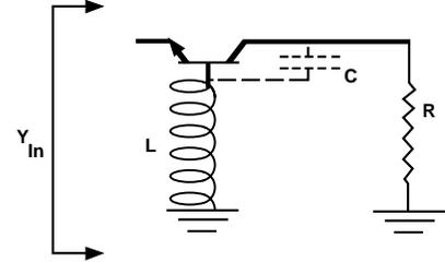
**Figure 4. When the designer adds a parallel resonant circuit to the equivalent circuit shown in Figure 2, the result is a complete voltage-controlled oscillator.**
