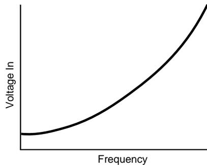
**Figure 15. Typical varactor-tuned-oscillator voltage-vs.-frequency curve. Note that, although nonlinear, the curve is monotonic—an increase in tuning voltage always results in an increase in frequency. This curve can be linearized with additional circuitry at the expense of new problems.**
