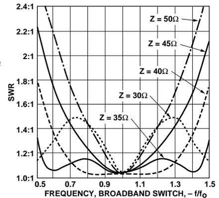
**Figure 5. SWR vs Frequency Ratio, Broadband Switch.**
