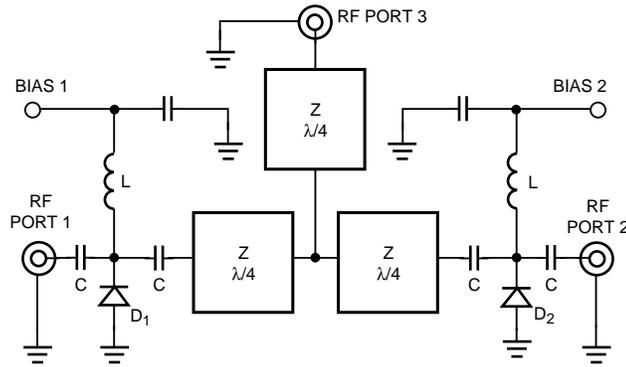
**Figure 4. Broadband Shunt SPDT Switch.**
